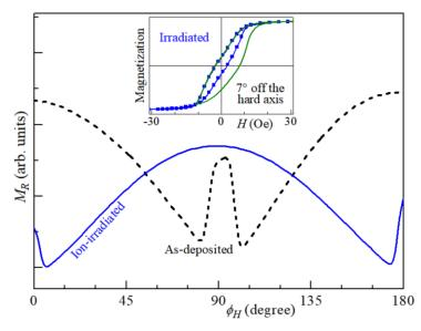
$M_R$  angular variations of both as-grown and Ne<sup>+</sup>-irradiated (70 keV, fluence of  $1\times10^{15}$  ions/cm<sup>2</sup>) 10-nm-thick Co films magnetron-sputtered on Si/Ta(18 nm). The inset shows a major (symbols) and a recoil magnetization loops of the irradiated film obtained for in-plane magnetic field applied 83° away from the (also in-plane) ion-irradiation-induced easy axis.
