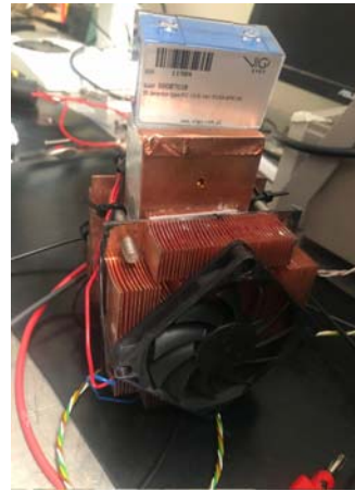
Fig.7. Final assembled detector cooled by Peltier cells ready to be tested.
