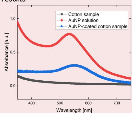
characterization in the UV-vis range of both solution and coated cotton reveals the presence of around 20 nm diameter Au NP associated to a peak at 550 nm.
