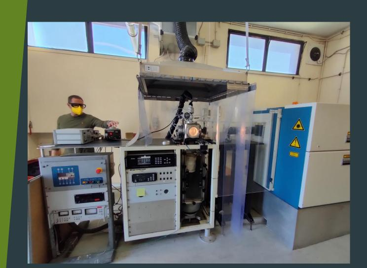
SiO<sub>2</sub> and TiO<sub>2</sub> nanoparticles were synthesized by using CO<sub>2</sub> laser pyrolysis of an aerosol of liquid precursors in a gas-flow reactor.
