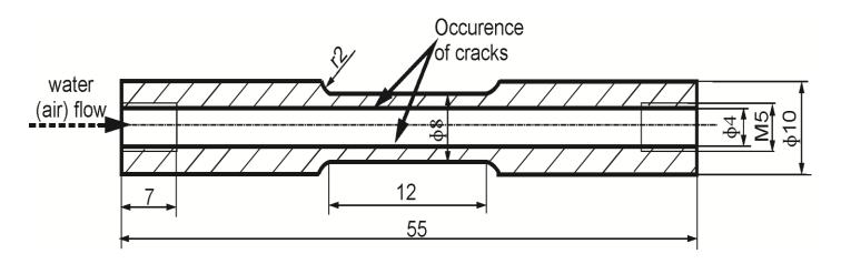
2. Specimen for testing of surface layer
