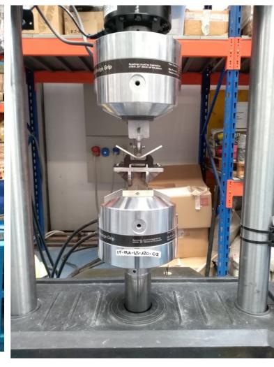
Commercial printing material (PLA) is tested, together with innovative nanocomposite. By production of a series of test samples, mechanical properties are characterized thought bend and tensile strength test. As a final step, the elements of the artifacts will be produced and the connection to the artworks is an additional key point for the success of the project.
