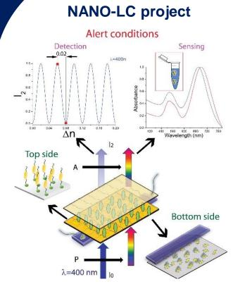
This work focuses on the fabrication and characterization of a label-free reusable localized surface plasmon resonance (LPSR) biosensor for the on-site detection of *Escherichia coli* cells in potable water.
